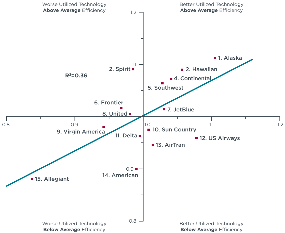
Figure 7. In-use fuel efficiency score (y-axis) versus normalized Technology Utilization Score (x-axis)
